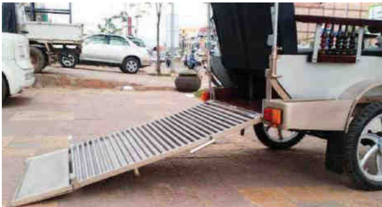
Figure 6.7. Accessible Mobilituk (Remork) with wheelchair ramp deployed (Research Team, 2020)
