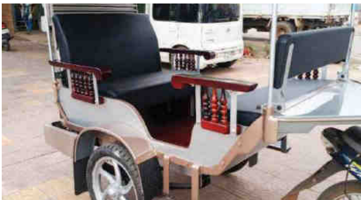
Figure 6.8. Accessible Mobilituk (Remork) in non-wheelchair mode. Note the sleek stainless steel construction complemented by traditional décor elements (Research Team, 2020)
