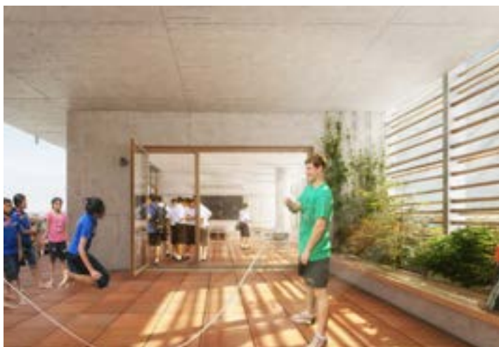
The open-air learning spaces are shaded with a bamboo screen, while other parts of the building use terracotta fins
