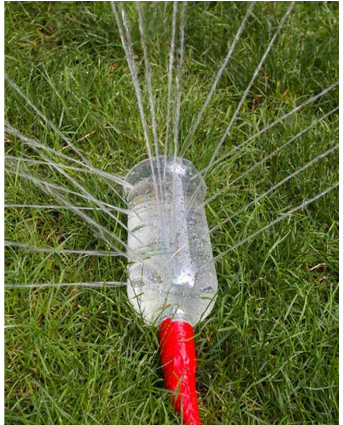
Sprinkler made from a water bottle
