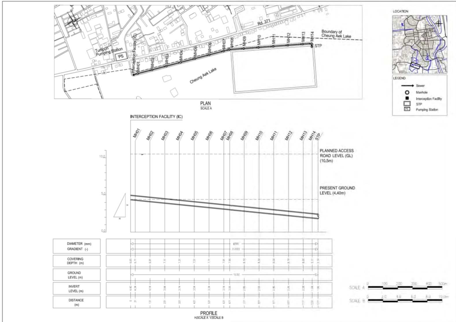
Fig. 8.2.1 Plan and Profile of Sewer Line in the Preparatory Project
