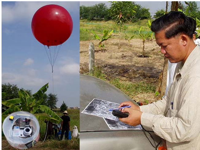
Figure 2: Digital aerial balloon photo technique
