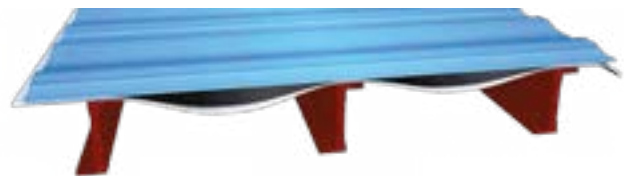
Roof insulation draped below metal sheet with air gap
