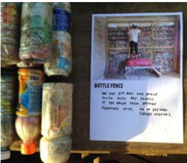
The Eco Blocks are bottles stuffed with plastic bags, polystyrene trays, straws.
