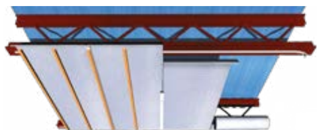
Roof insulation below rafters as retrofit solution
