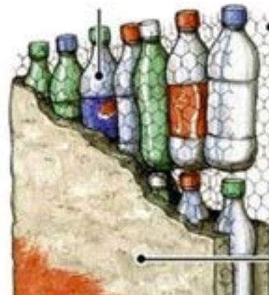
Layers of plastic bottle wall
