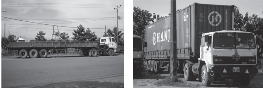
Figure 2.3-7 Flat-body truck without twist lock pins
