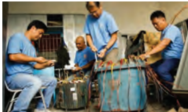
Rewinding well-pump motors
